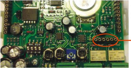
Version with PoE compatibile only with VoIP modules with 6 pin connector
