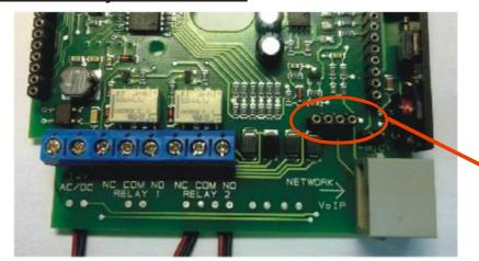
Version with PoE compatibile only with VoIP modules with added 2 wires on top board of VoIP module
