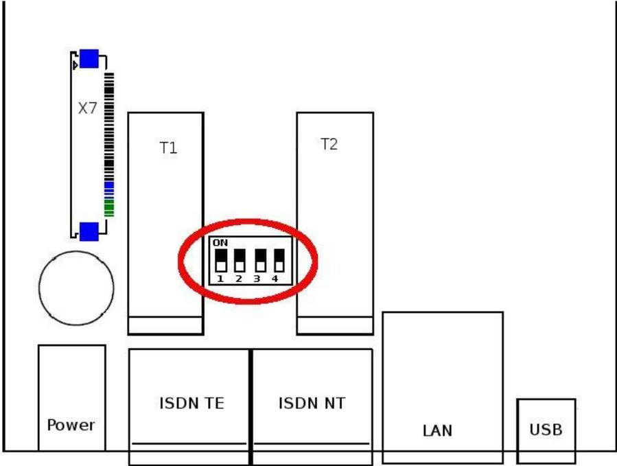
Picture 3: Setting for Router or TE mode
