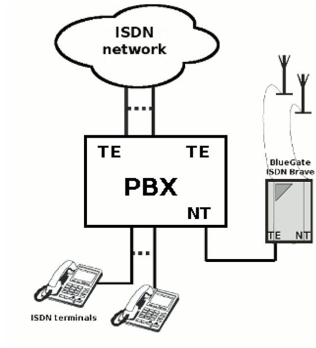
*Picture 5: Connection of the Blue Gate ISDN Brave in TE mode.*
