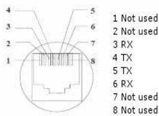
Fig.: contacts of NT connectors
