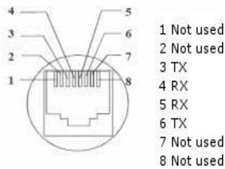
Fig.: contacts of TE connectors
