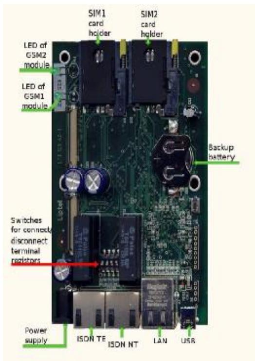
It is necessary to check whether the terminal resistors So of the bus (100R) are in the socket.
