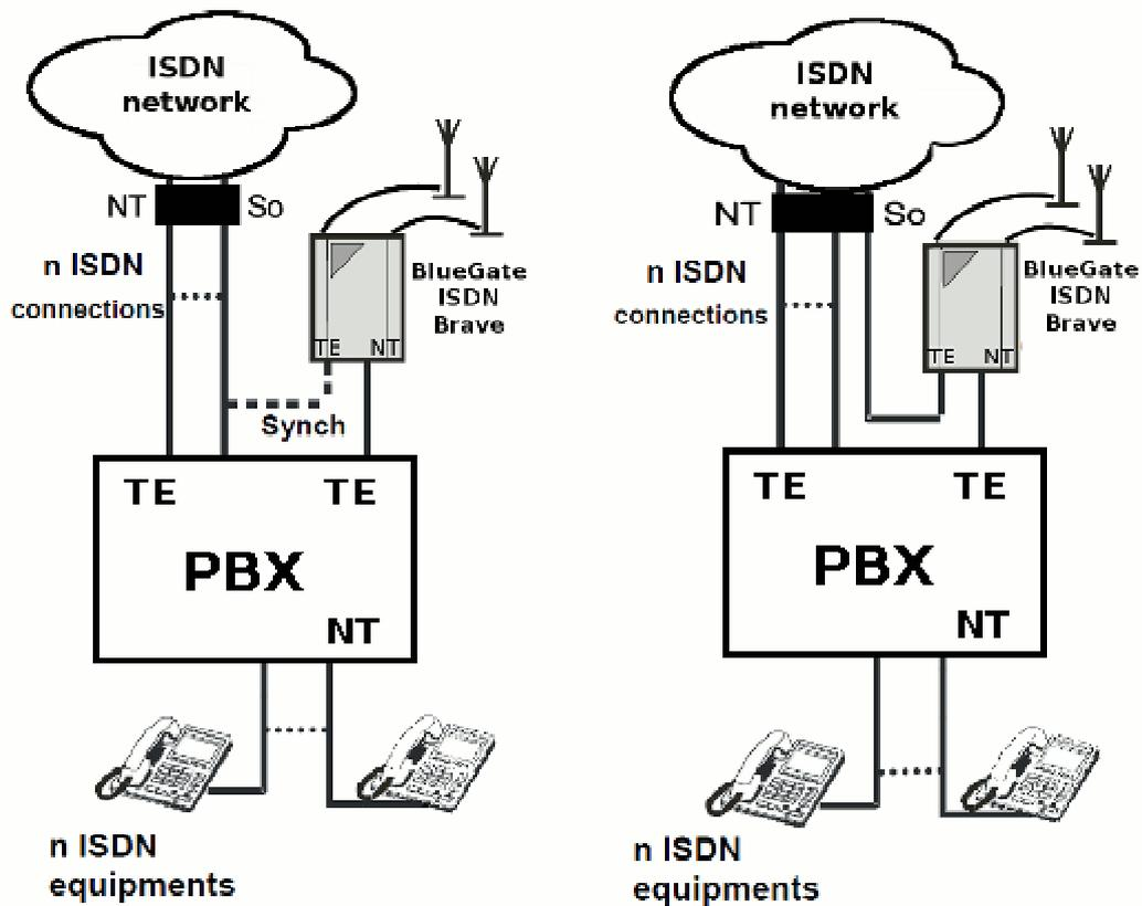
Picture 4: Connection of the Blue Gate ISDN Brave in the SYNCHRO mode and as the ROUTER.
